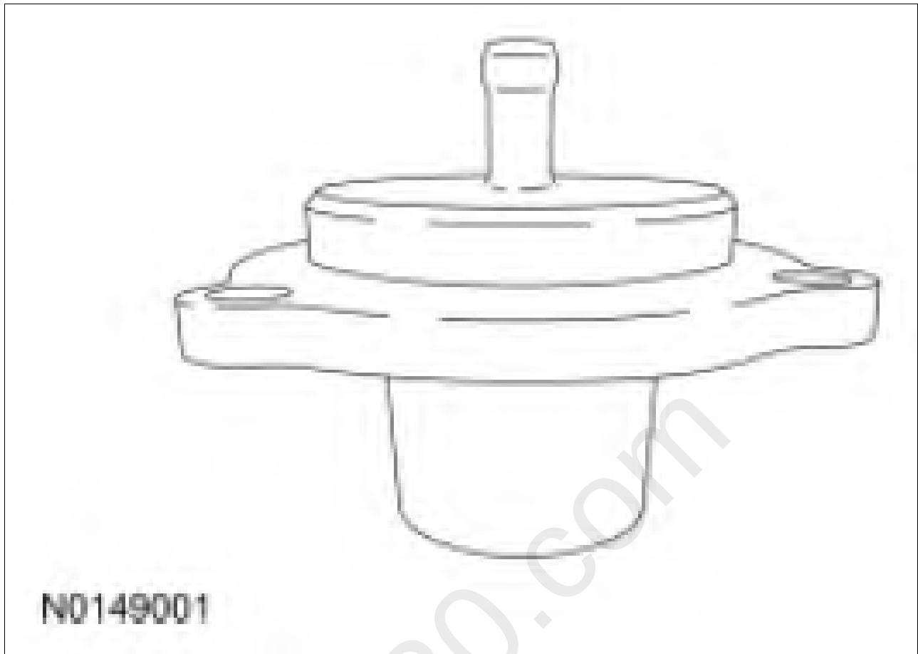
Fig 2: Identifying Turbocharger Bypass Valve (Pneumatic Control)
